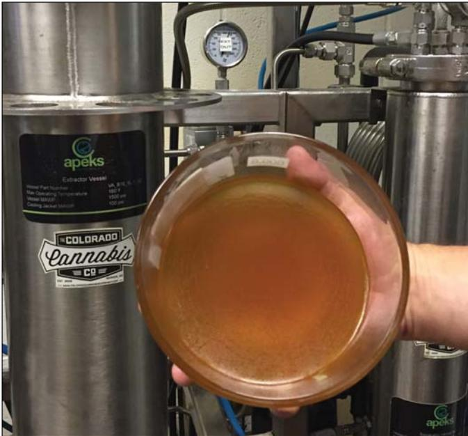
Cold separation processes protect plant oils resulting in higher-quality extractions like this one from the Colorado Cannabis Company in Denver.
