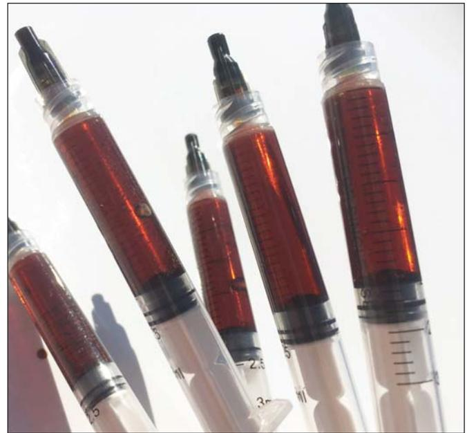
Using an Apeks 2000psi CO<sub>2</sub> extraction system utilizing cold separation, SJR Labs in Gorham, Maine was able to offer 78% THC pure amber cannabis oil in these 2g syringes.
