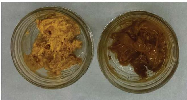
**Greater consistency; higher potency.** The lighter, purer extraction on the left is the result of cold separation processing. The darkened extraction from the very same extractor without using cold separation has been thermally degraded by high temperatures in the separator vessel.
